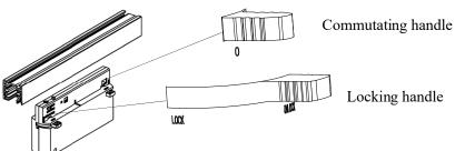
2. Align the boss of the guide light connector with the groove of the guide rail before assembly.
