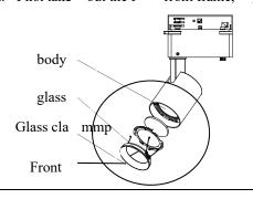
Removve the glass press plate by turni ng it in thh e direcction of the arrowas shown
