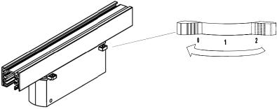
2. Then turn the LOCK handle counterclockwise to switch from "LOCK" to "UNLOCK".
