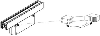
3. Finally, pull down one end of the guide light connector to remove the entire guide light connector.
